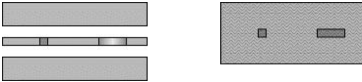
Figure 1. Polyguide(tm) single mode exposure process steps. Both primary and secondary diffusion are important for creating a robust film structure and uniform guides of different widths. Waveguide and buffer / clad layers are identical. Typically, exposure power is 14mW/cmsq. and energy is 100mJ/cmsq. Standard light box mercury arcs are used. Baking is usually at 135°C for 2 hours. Exposure temperatures are varied to produce different guide indices.
