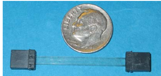
Figure 1. 8x8 Star Coupler with MT ferrules
