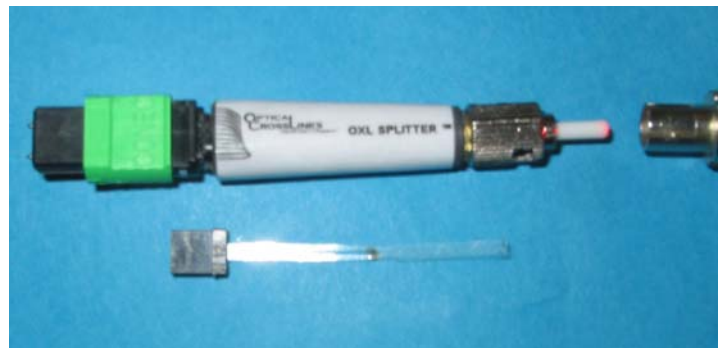
Figure 1: Component packaged 1x16 splitter with flexible connector housings; and special board unit
