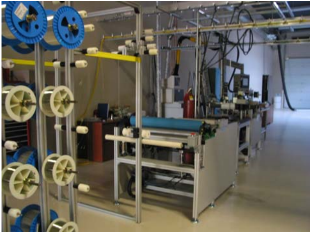
Figure 3 (above) Production Apparatus Facility for fiber ribbonization and shuffle creation, including fiber creels, tension control, ribbon forming die, ink jet printer for ribbon and fiber identification, and UV cure and workstations
